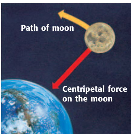
Figure 8 The moon stays in orbit around the Earth because Earth's gravitational force provides a centripetal force on the moon.
